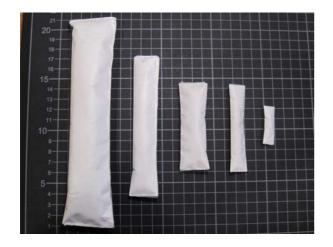
EZ•DRY Moisture Traps are used for efficient removal of water from solvents and reagents. The traps will maintain anhydrous conditions of 30 ppm or less while resisting increases in water content due to routine or repeated opening of reagent containers.
