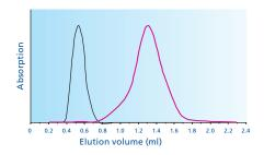
Elution profile overlay of 0.1 µmol 5-TAMRA and 0.04 µmol oligonucleotide (200 µl sample volume).
