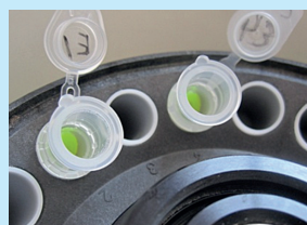
Figure 1 Orientation mark on column is aligned upward for storage buffer elution.
