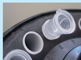
Figure 3 Orientation marks are aligned upward for sample elution.
